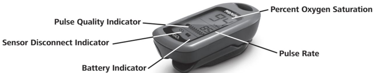
The Battery indicator symbol
